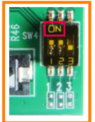
SW4 SETUP - NVMe SSD & SAS / SATA device switch
