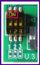
SW2 SETUP - NVMe SSD & SAS / SATA device switch
